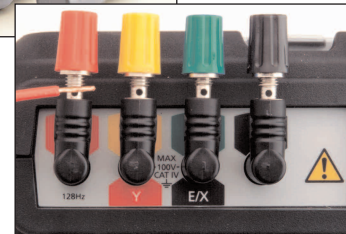
Terminal Adapters are optional accessories used to allow the units' terminals to accept alternative cable connections.
