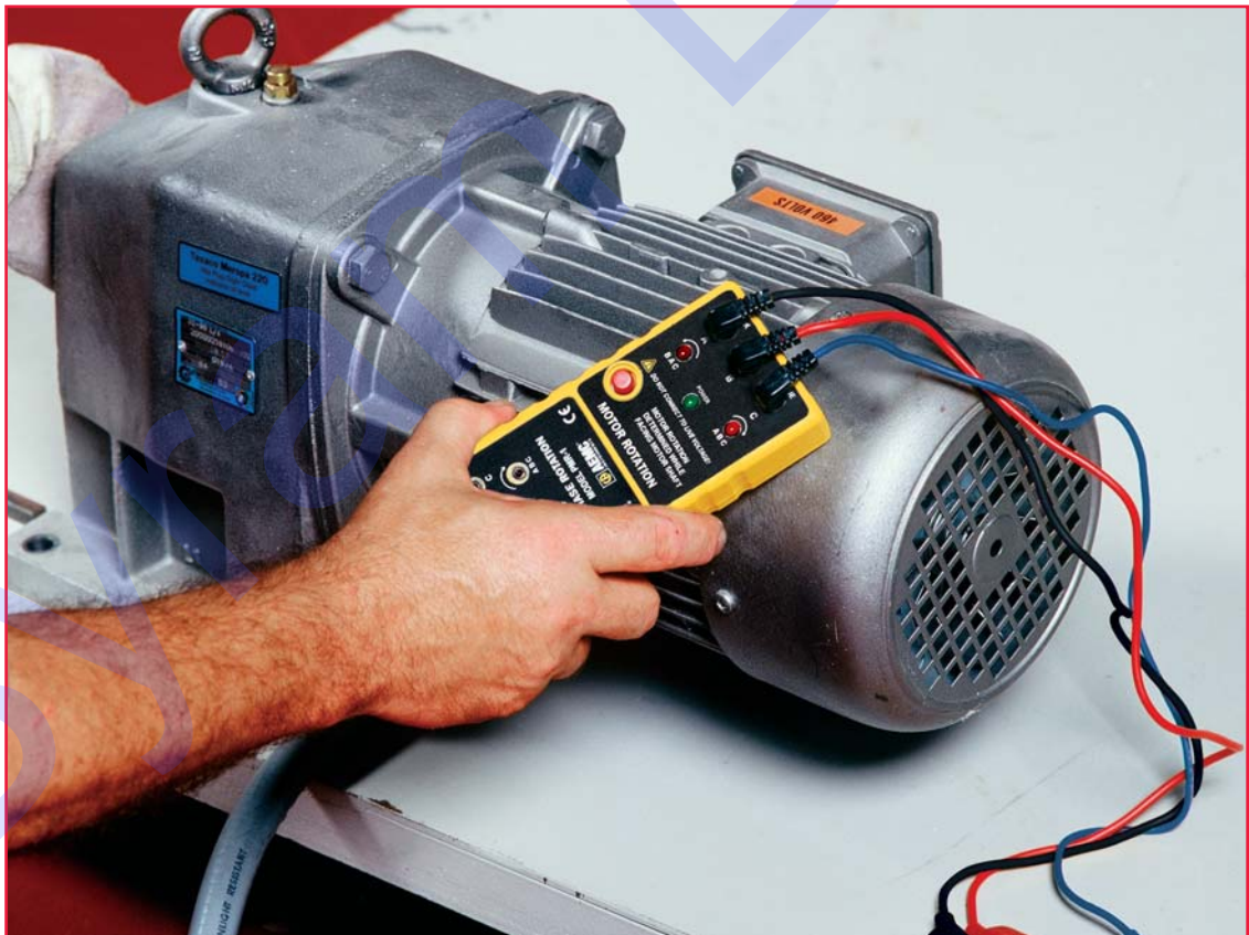
Phase and Motor Rotation Tester Model PMR-1 verifying motor rotation.
